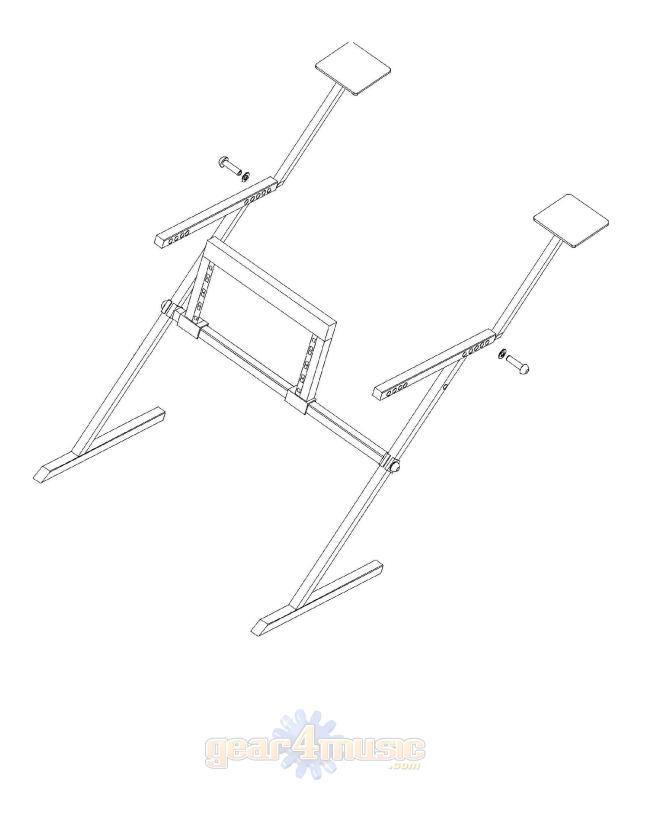
6) Fix the two small shelf brackets to the lower support bar as illustrated below.
