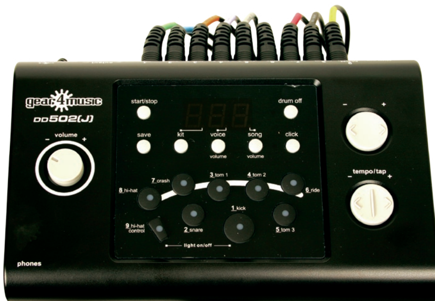
▲ The DD502-J 'brain' holds 20 preset kits and 10 user kits, comprising 215 individual sounds.
