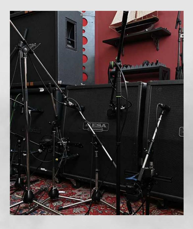
To put it simply, an impulse response is a capture of the speaker cabinet, the microphone, preamp, and any other gear in the recording chain.
