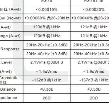
**Note: The above data is the result of the test in TOPPING laboratory.**
