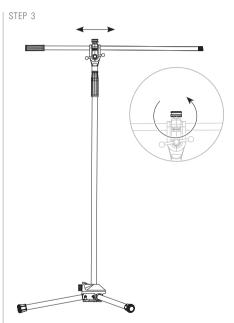
Adjust the boom arm to desired position using the knob.
