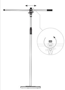
Adjust the boom arm to desired position using the two knobs.
