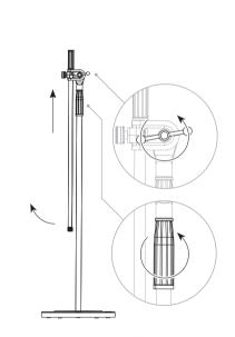
Loosen the boom arm clutch and position the arm to desired angle. Re-tighten the boom arm clutch. Adjust the height to desired position using the central collar.
