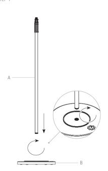
Attach the pole (A) to the base (B) and screw into place.
