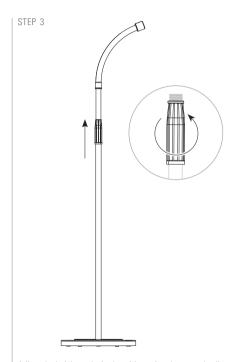
Adjust the height to desired position using the central collar.
