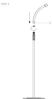
Attach the goose neck (C) to the pole (A) and screw into place.
