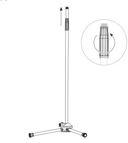
Adjust the height to desired position using the central collar.
