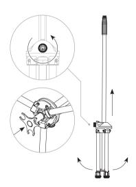
Loosen the knob and detach the legs from the leg clip. Move the three legs into the fully open position and lift the centre pole up. Re-tighten the knob and push the clip into the bottom of the base.
