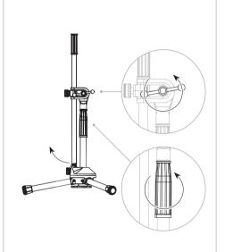
Loosen the boom arm clutch and position the arm to desired angle. Re-tighten the boom arm clutch. Adjust the height to desired position using the central collar.
