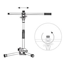
Adjust the boom arm to desired position using the knob.
