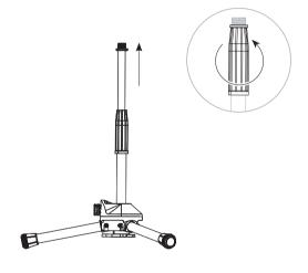
Adjust the height to desired position using the central collar.
