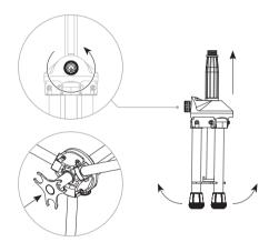
Loosen the knob and detach the legs from the leg clip. Move the three legs into the fully open position and lift the centre pole up. Re-tighten the knob and push the clip into the bottom of the base.
