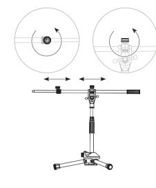
Adjust the boom arm to desired position using the two knobs.
