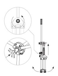
Loosen the knob and detach the legs from the leg clip. Move the three legs into the fully open position and lift the centre pole up. Re-tighten the knob and push the clip into the bottom of the base.
