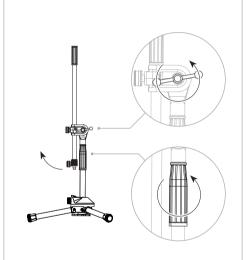
Loosen the boom arm clutch and position the arm to desired angle. Re-tighten the boom arm clutch. Adjust the height to desired position using the central collar.
