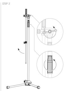
Loosen the boom arm clutch and position the arm to desired angle. Re-tighten the boom arm clutch. Adjust the height to desired position using the central collar.
