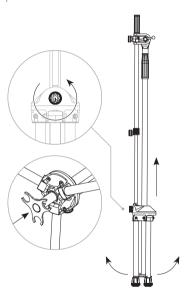
Loosen the knob and detach the legs from the leg clip. Move the three legs into the fully open position and lift the centre pole up. Re-tighten the knob and push the clip into the bottom of the base.
