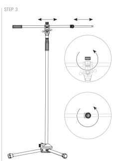
Adjust the boom arm to desired position using the two knobs.
