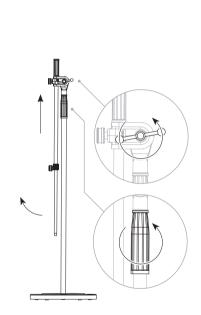
Loosen the boom arm clutch and position the arm to desired angle. Re-tighten the boom arm clutch. Adjust the height to desired position using the central collar.
