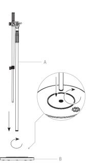
Attach the pole (A) to the base (B) and screw to fix into place.
