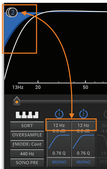
Figure 6 — Two cascaded Sections with the "same" apparent setting and differing actual frequencies
