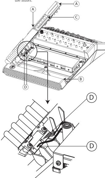
5. At this point, your goal is to remove the current iPad dock assembly from the tray assembly and replace it with the Lightning iPad dock assembly included with this kit.
