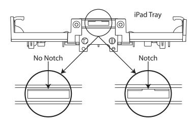
8. Your tray does not have a notch, but that's ok. You can make one by following the steps listed below. The notch is for clearing room for the connector to fit, so neatness of the slot is not overly critical. You cannot hurt the function of the part by oversizing the notch slightly. Additionally, the notch will be covered, hiding any blemishes.
