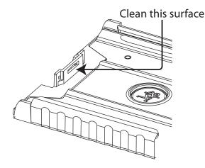
10. Let's put it back together. Insert the new Lightning dock subassembly into the tray. Using the #1 Phillips screwdriver, secure the assembly to the tray assembly by reattaching the two machine screws and two plastic threading screws to the same places from where they were removed in step 5.
