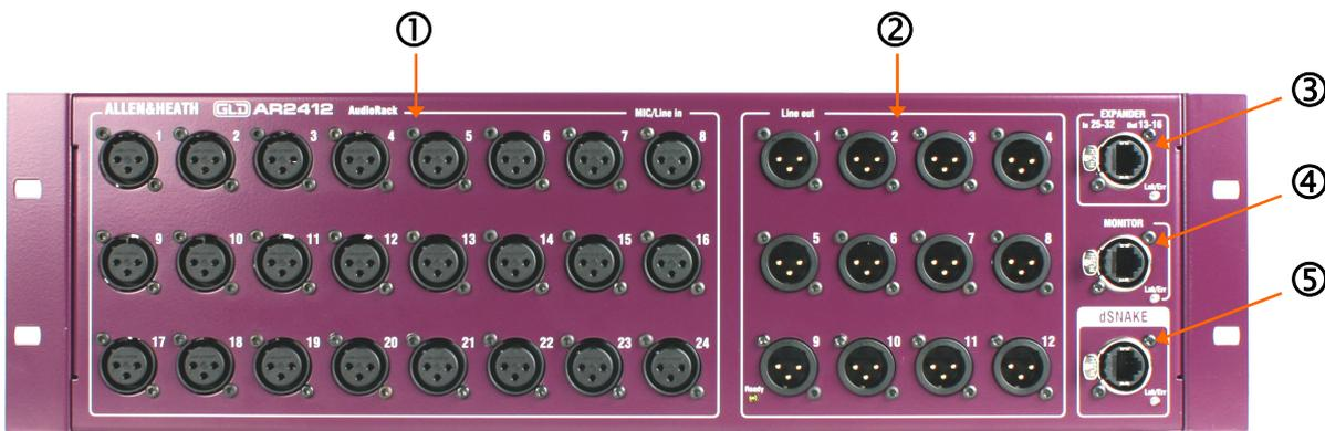
**① Input sockets** 24 balanced XLR inputs for microphone and line level sources. The preamps are built into the AR2412 rack and their Gain, Pad and 48V phantom power is remote controlled from the GLD console via the dSNAKE link. The output of the analogue preamps are converted to digital format and transported via dSNAKE to be processed and mixed at the GLD-80 mixer.
