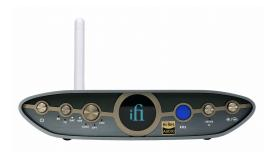
The ZEN Blue 3 is the world's first DAC wirelessly receive and transmit Lossless Bluetooth audio. It delivers exceptional hi-res wireless audio, courtesy of Qualcomm's QCC518x Bluetooth audio chip and the aptX Lossless codec.
