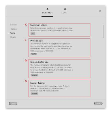
$\underline{\text{N. MASTER TUNING}}$  The default tuning (in Hz) of the A above middle C.
