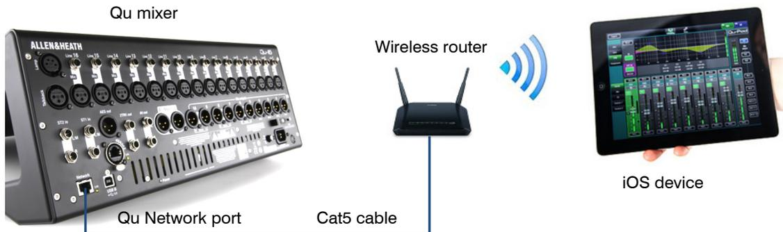
**Choosing a wireless router** - For best performance use a dual band (2.4 and 5GHz) wireless router (wireless access point) with auto channel selection.
