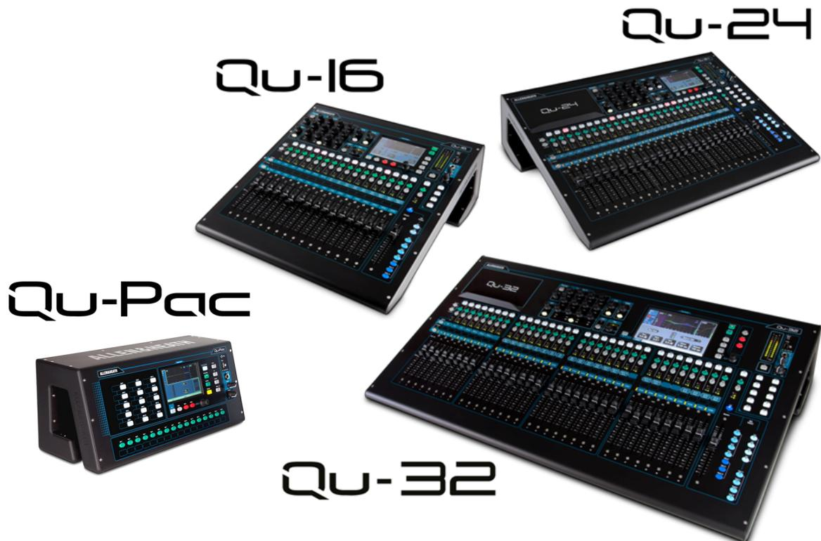
Qu-Pac is part of the Allen & Heath Qu Series of digital mixers. It is a faderless version with the same local connections as the Qu-16, but features the Qu-32 mix engine and can therefore be expanded to 32 channels using an optional AudioRack linked via the dSNAKE Cat5 digital snake. Qu-Pac is intended for wireless live mixing, for example using an iPad. It can also be fully controlled using its front panel touch screen. Qu-Pac has many applications where a compact solution is required:
