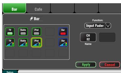
Functions can be assigned to up to 15 positions arranged as a grid of 3 rows with 5 columns. If a position is unassigned then it will appear blank in the user screen.
