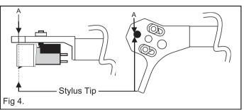
Should the stylus need replacement it can be removed by pulling the white coloured front section away from the cartridge body.
