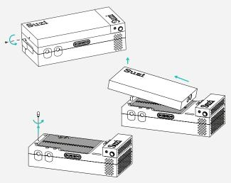
Carefully place a connecting unit on top of the Suzi power amp and ensure they are aligned. Gently slide the partnering device towards the Suzi to connect any (female) outputs to Suzi's (male) inputs.
