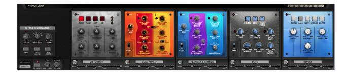
This supplements the controls under the keyboard with detailed parameters for each of the five **Effects** processors.
