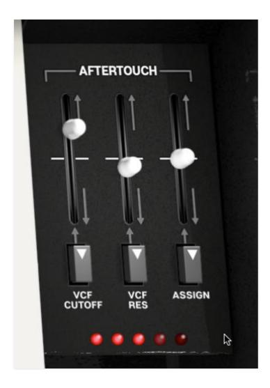
**Aftertouch** is a term coined by Yamaha to describe the touch sensitivity of its earliest synthesizers. They used the names *initial touch* for velocity and *after touch* for what was commonly called *pressure*. The massive popularity of the Yamaha DX7 led to the word "aftertouch" becoming the most popular generic name for this type of modulation control.
