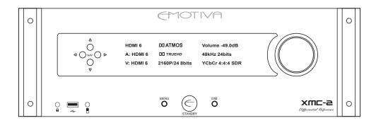
The front panel of the XMC-2+ is dominated by a large, bright, easy to read blue OLED display. The display can be set to any of six different brightness levels, including totally off. If the display is fully dimmed, it will illuminate for a few seconds when you press the Info button, and, when you activate the Menu, the display will illuminate for as long as you are using the Menu.
