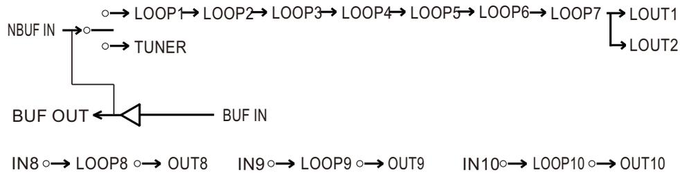
Guitar signal feeds into OC10 input (NBUF IN or BUF IN), enters series LOOP1~LOOP7 when MUTE switch is off, then outputs from OUT-1 and OUT-2. when TUNER switch is pushed, the signal outputs to TUNER jack. Be noted the BUF OUT jack doesn't output when the guitar plug into NBUF IN jack.
