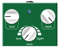
Ambient Texture (Sounds Amazing With Faux Tape Echo!) Level at 9 o'clock, Depth fully clockwise, Shade fully counterclockwise
