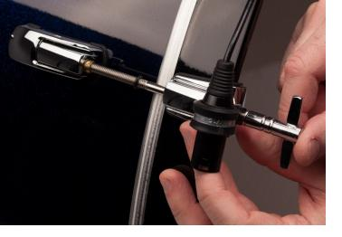
**6.** Connect the DrumLite Controller to the DrumLite LED connector. Carefully connect them without bending the five pins.
