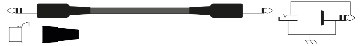
TS-to-TRS Adapter (ring not connected)
