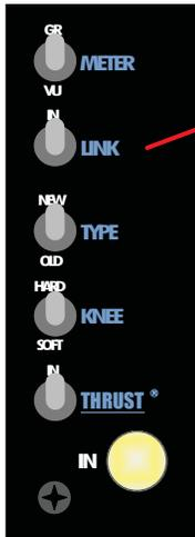
LINK: The LINK switch activates the DC control voltage summing with other units.
