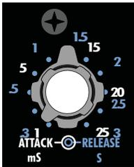
Attack and Release times are fully variable on the 527 Compressor and share a dual-concentric potentiometer for control. Attack time is adjusted using the outer ring of the pot and Release time is adjusted using the inner knob.
