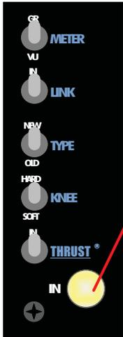
IN: The In/OUT switch inserts or removes the 527 from the audio path via a relay bypass. When the switch is in the OUT position, a relay connects the audio Input to the Output – completely removing the 527 from the audio chain.
