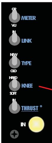
Knee determines the 527 Compressor's response curve at the onset of compression.
