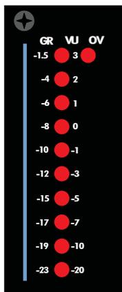
An **OUT**put level meter is provided to indicate the 527's output in VU when the METER switch is in the VU position.
