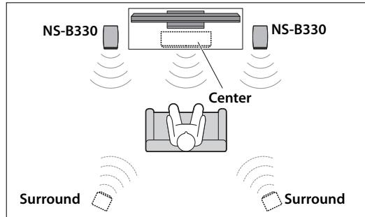
Position the speakers on both sides of the TV. The positioning of speakers is important, since this dictates the overall sound quality of the multi-channel system. Set up the speakers on the basis of your listening position by following the owner's manual supplied with your amplifier.
