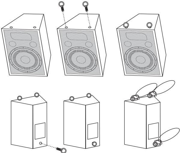
**Please note:** Before installing the eye bolts, make sure that the thread is is always in perfect condition and free from dirt.
