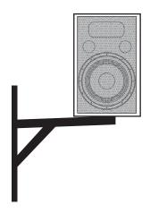
Before attaching the speaker system, make sure that the installation area can hold a minimum point load of 10 times the installations weight. (e.g. 13Kgs - 130Kgs point load).
