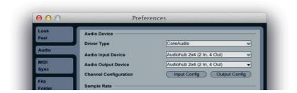
Once the Audiohub 2x4 is set as the preferred Audio Device\* in your DAW, its inputs (1 and 2), and outputs (1 to 4), will appear in your DAW's Audio I/O preferences. Depending on your DAW, you may need to enable certain inputs or outputs before use. The two examples below show Inputs 1 and 2 and Outputs 1 to 4 enabled in the Ableton Lite Audio Preferences.
