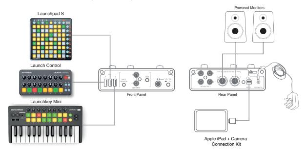
Note that the Audiohub 2x4's hub function is always available to link USB devices into your computer or iPad, regardless of how you use the audio I/O section. The three examples which follow demonstrate how you can also link analogue audio into your system.
