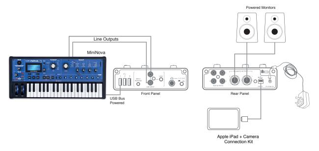
Connect the synth's audio output to the Audiohub 2x4's LINE INPUT phono (RCA) sockets. Connect either **BALANCED OUTPUTS 1** and **2** or **RCA OUTPUTS 1** and **2** to your powered monitor speakers (depending what type of inputs they have) with appropriate cables (see "Connecting speakers" on page 17).
