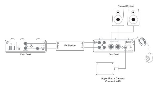
You can use Audiohub 2x4 to create a send/return loop to add an external FX processor into your system. Because the Audiohub 2x4 has two pairs of outputs, you can use **RCA OUTPUTS** 3 and 4 to feed the inputs of the processor (output selection made from your DAW) while using **BALANCED OUTPUTS** (or **RCA OUTPUTS**) 1 and 2 for monitoring. The outputs of the processor are connected back to the Audiohub's **LINE INPUT**s.
