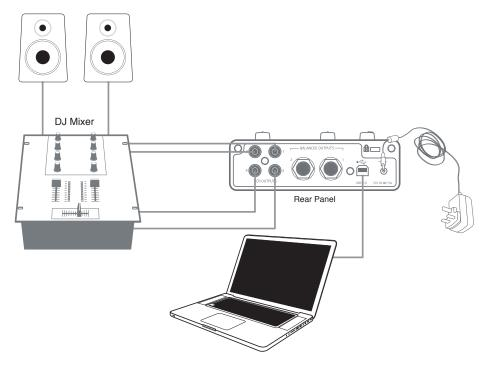
The Audiohub 2x4 can be used as an interface between a laptop running DJ software and the channels of a DJ mixer. In this setup, Outputs 1 and 2 can be connected to Line Inputs 1 and 2 of an external DJ mixer, and Outputs 3 and 4 to Line Inputs 3 and 4. Connecting in this way means that all mixer facilities, such as EQs and crossfading, are easily accessible.
