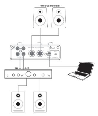
Self-powered monitors (i.e., typical computer speakers) incorporate internal amplifiers with a volume control, and may be connected directly to the Audiohub's outputs. Larger, passive loudspeakers will require a separate stereo amplifier; in this case, the outputs should be connected to the amplifier's inputs.
