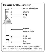
Fig. 4.2: TRS stereo connector
