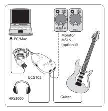
Fig. 3.1: Wiring of the UCG102
