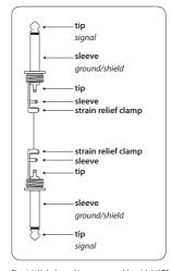
Fig. 4.1: Unbalanced instrument cable with  $\frac{1}{4}$ " TS connector
