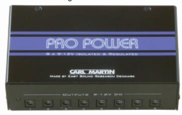
Start with the switchable (110-230 V) fused AC input, and split that into 8 individual isolated and regulated 9v (100mA) – 12v (90mA) outputs, with extended power at output 7-8
