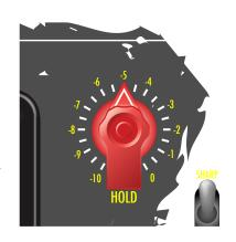
NOTE: The 'HOLD' control works independently of input level applied to the compressor/limiter.
