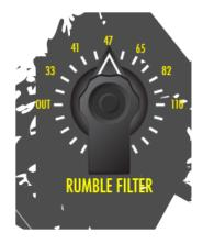
The 'RUMBLE FILTER' control is a low cut mechanism, featuring six frequency settings (33, 41, 47, 65, 82, 110hz.) The 'RUMBLE FILTER' may be fully disengaged from the amplifier by setting it to 'OUT.' This feature is useful for removing unwanted low frequency information from the signal.
