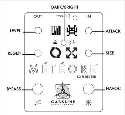
ATTACK sets the amount of gain in the preamp, allowing you to boost or overdrive the reverb. SIZE establishes the inital reverberation. REGENERATION extends the decay and adds overtones; set both this and SIZE high and the pedal can run away and self oscillate. LEVEL is the overall volume of the effect relative to your original signal. The DARK/BRIGHT toggle sets the overall voice.
