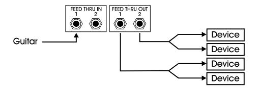
Because GCX feed thru's have low impedance outputs, you can drive multiple devices from each output. In this example, the guitar signal passes to all four devices using two Y-cables.
