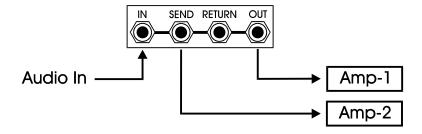
When the loop is OFF, Amp-1 plays. When the loop is ON, Amp-2 plays.
