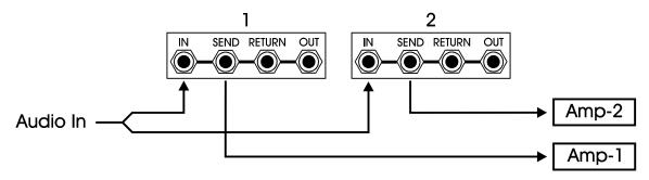
When loop #1 is ON and loop #2 is OFF, only Amp-1 is active. With loop #1 OFF and loop #2 ON, only Amp-2 is active. When both loops are ON, both amps play at the same time.
