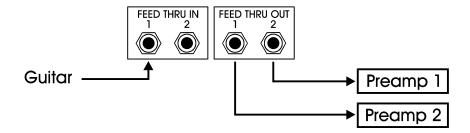
Since the two feed thru's are normalled together, the guitar signal passes from GUITAR IN to both GUITAR OUT and FEED THRU.
