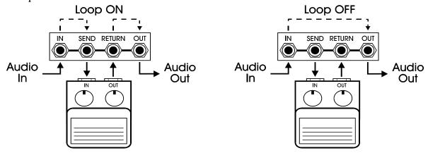
In this example, when the loop is ON, the pedal is active. When the loop is OFF, the pedal is bypassed.
