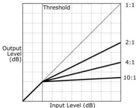
The **ratio** determines how much gain reduction will be applied to the signal once it crosses the threshold. At a 4:1 ratio, for every 4dB of input signal above the threshold, there will be 1dB of output signal. A 10:1 ratio would output 1dB for every 10dB of input signal, etc.
