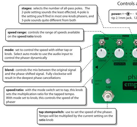
\* these controls are for tap and knob modes. Auto mode uses the control
