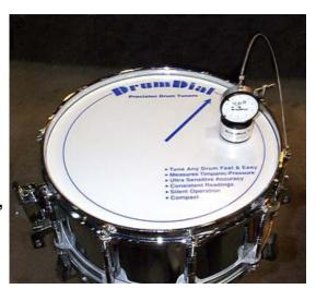
You can eliminate these problems by using a Drum Dial to measure drumhead tension directly from the drumhead, allowing you to precisely tune your drums faster and easier than ever before. Drum Dial has been designed and manufactured to the highest quality standards with all the key features you would expect from the best drum tuner available. Get the tuner that really works, get a Drum Dial and make it possible for your drums to consistently sound great!
