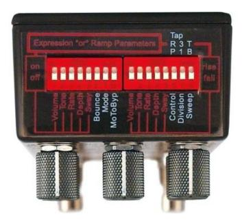
A very important thing to remember is that ramping always gets reset when bypassing. The parameters' current knob position control where the parameters ultimately will either start or stop ramping.
