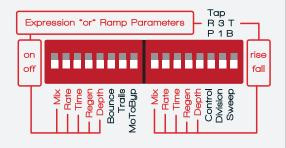
A very important thing to remember is that ramping always gets reset when bypassing. The parameters' current knob position control where the parameters ultimately will either start or stop ramping.
