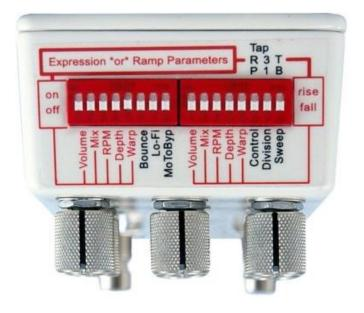
A very important thing to remember is that ramping always gets reset when bypassing. The parameters' current knob position control where the parameters ultimately will either start or stop ramping.
