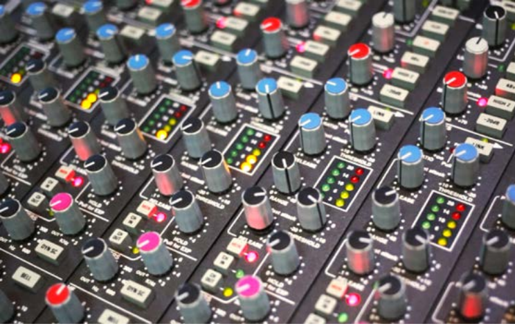
XL 9000 K compressor section.
