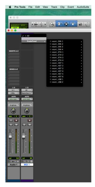
Note: After changing a port name in iConfig, it may be necessary to remove the mio4 from the computer's device listing and re-connect the mio4 so that the computer refreshes the port name.
