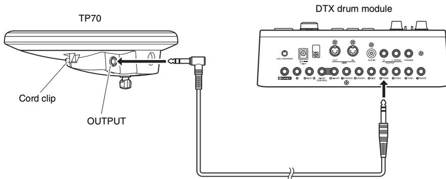
**NOTE** In order to protect both the cable and the jack from damage, be sure to hook the cable around the cord clip.
