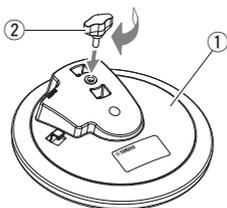
2. Slide the drum pad ① onto the hexagonal tom holder ③ from the rack or tom stand, and then tighten the S wing bolt ② to secure it in place.
