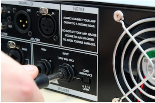
Then, plug that cable into the "SPEAKER INPUT" jack input of the *Torpedo Studio* (number 12 in figure 3.2).
