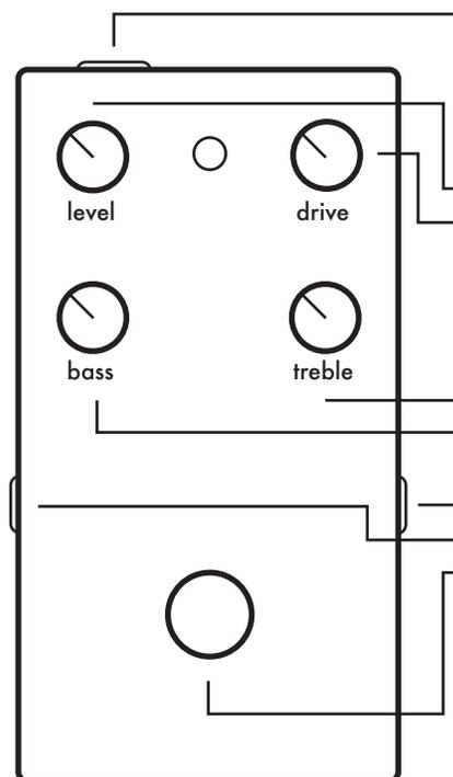
**Power** - Internal 9-volt battery or external DC 9 volt power supply is activated by plugging a cable into the input. The input cable should be removed when the unit is not in use to avoid running down the battery.
