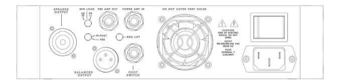
Use a regular mono instrument cable to connect the amplifier to the footswitch.
