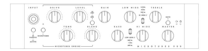
**GAIN**: Changes the volume of the signal the Active 4 Band EQ. You can set it low prior to ensuring the cleanest operation possible or set it higher for more aggressive growl.
