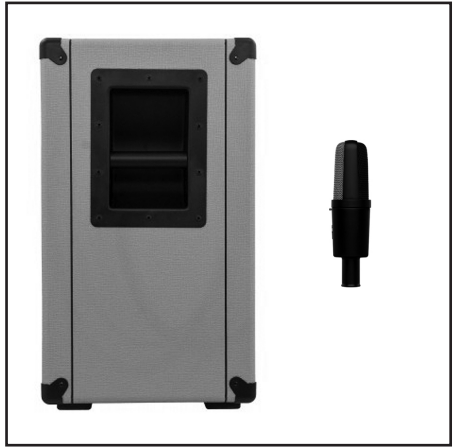
A WA-14 placed 6-8 inches from the speaker cone of a 4x12 guitar cabinet.
